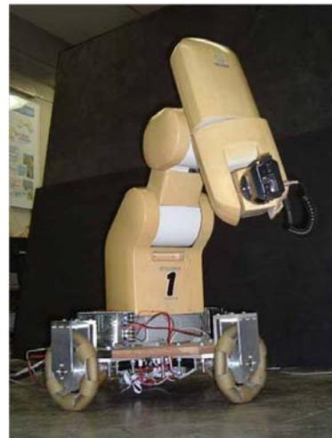
Figure 2 Developed mobile manipulator
