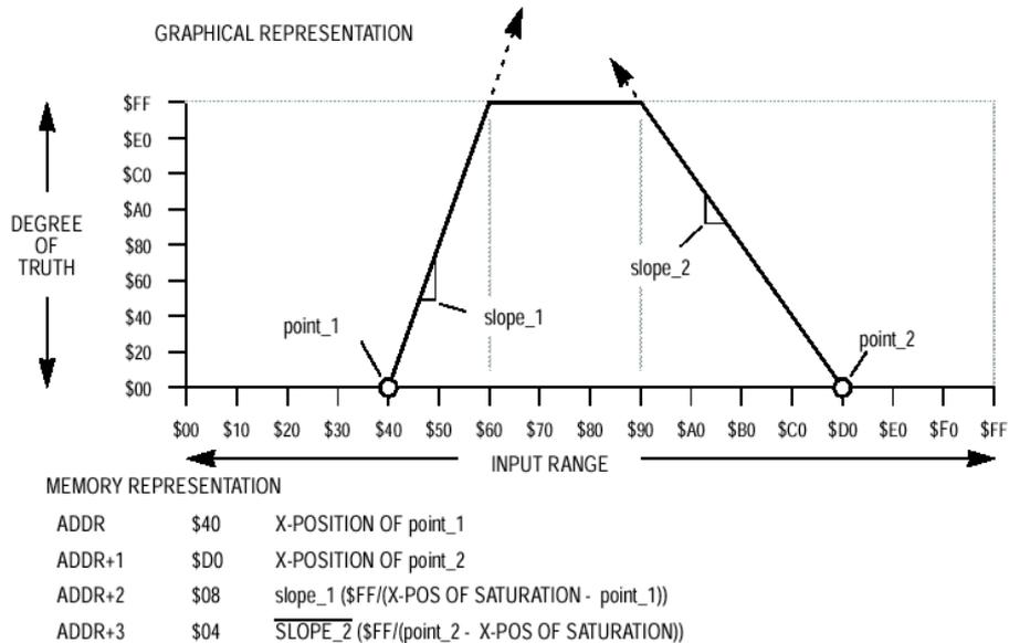
**Fig 3:** Trapezoidal membership function. The x-axis represents the input range and the y-axis represents the truth degree [5].
