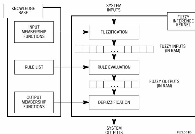
Fig2. Block diagram of a fuzzy logic system [6].
