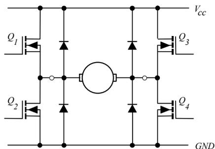
**Figure 5.** Wiring of motor supply
