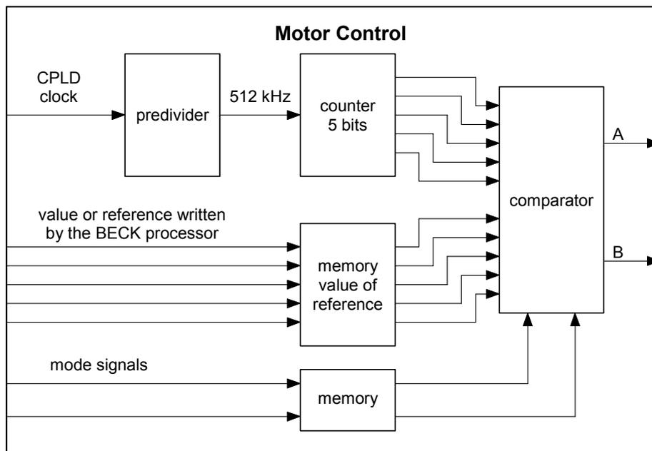
Figure 7. Motor control architecture
