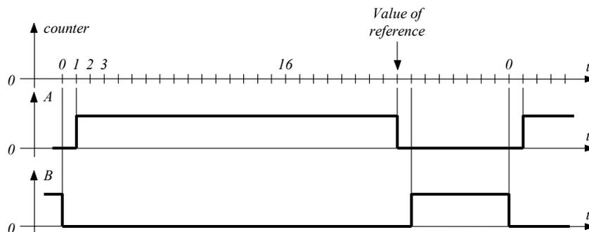
Figure 8. A and B control signals
