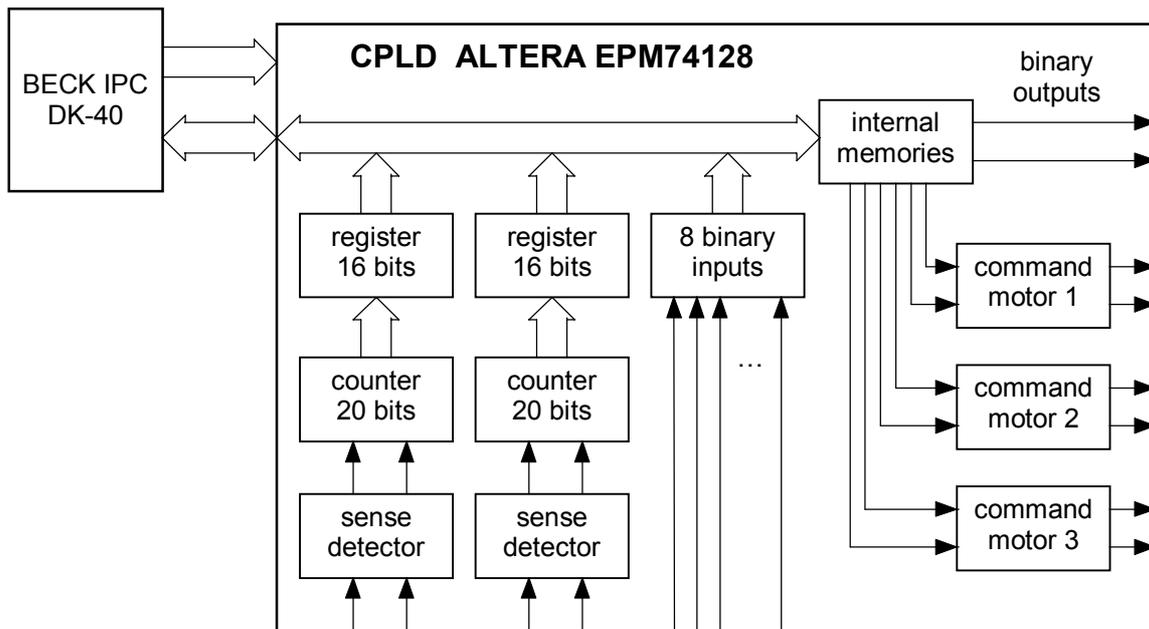
**Figure 4.** Schematic diagram of CPLD board
